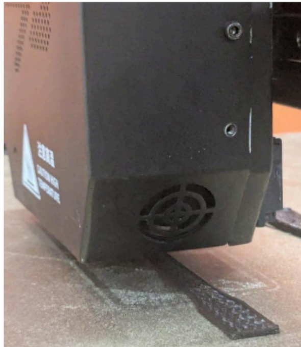
Fig 3.8: Piocreat G5 Ultra single screw extrusion printer printing ASTM sample
