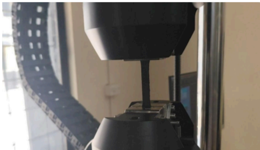
Fig 4.1: ASTM sample in UTM machine
