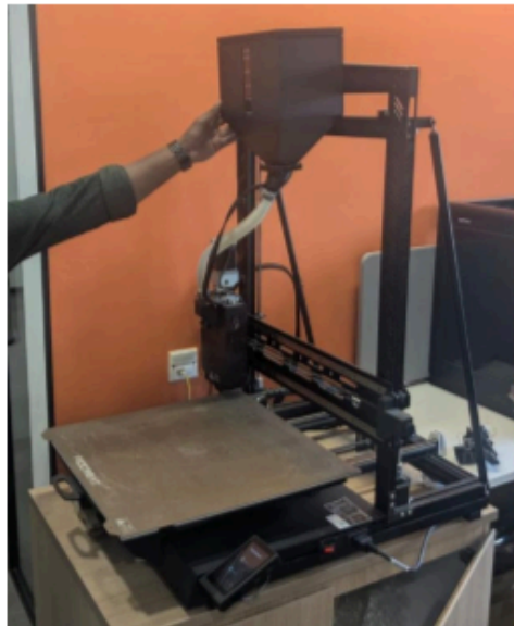
Fig 3.7: Piocreat G5 Ultra single screw extrusion printer
